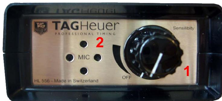
1. Sensitivity potentiometer with ON/OFF switch
