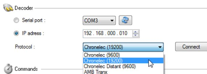
Select the Serial Port or Ethernet connexion. Several Protocols are available:
