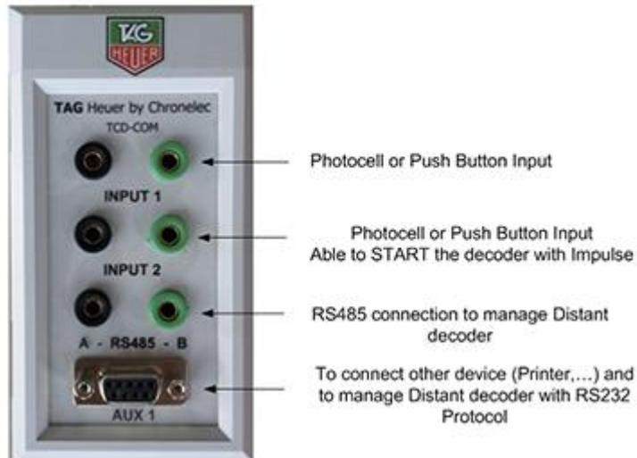
Example with connection between Distant and Master decoder
